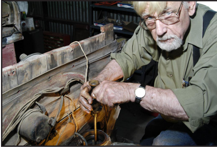
Above: 1920 Seagrave fire truck in the Duarte Garage. (Bill Nale photo) Below: Chuck Mcfann working on the exhaust valves of the engine. (Irv Stowers photo)
