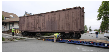
Above: Workmen cut welds that hold the car to the tracks. Photo by Jeff Kaskey. Below: the car moves onto the trailer. Photo by Bill Nale.
