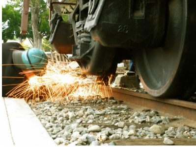
Above: Workmen cut welds that hold the car to the tracks. Photo by Jeff Kaskey. Below: the car moves onto the trailer. Photo by Bill Nale.
