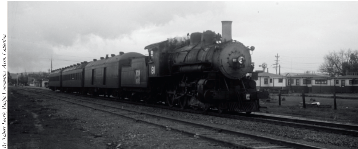
WP Feather River Express passes west-bound through Livermore on April 20, 1947. Locomotive No. 81 (ten-wheeler, 4-6-0) is followed by a tender, a baggage car and two passenger coaches.
