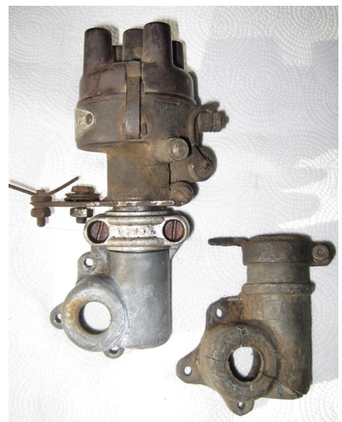
Above: Frank Duarte; photo donated by Bernice Myers. Left: The distributor from the Star engine donated by Curtis Freih. The casting at the right end is pot metal, usually composed mostly of zinc, which can creak and deteriorate with age. Photo by Will Bolton. Below: On the left of the photo is the Star distributor mounted on the newer casting donated by Bert Babick. The old, badly deteriorated casting is shown on the right. Photo by Will Bolton.
