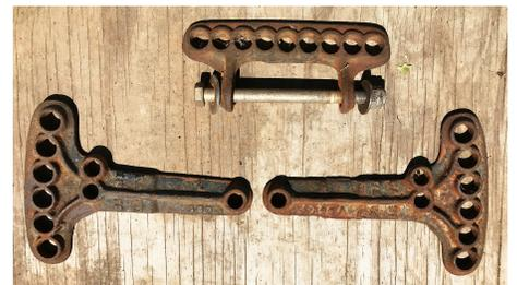
Above: Identification complete! The various parts of a clevis hitch. Photo by Jeff Kaskey
